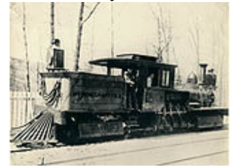
One of the two Shaygeared Locomotives that moved the cars up the mountain until 1898 when the Gravity Railroad was electrified. Photo courtesy BCHS website.
